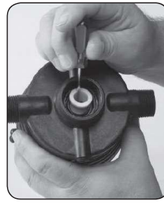
Step 3. Remove #83 SHAFT SEAL SPACER.
