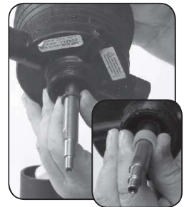
Step 6. Remove and replace #17 O-ring, Re-install #83 SHAFT SEAL SPACER and #15 SEAL RETAINER.
