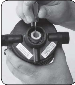
Step 4. Remove #82 SHAFT SEAL SPACER.
