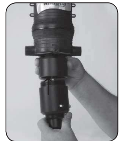
Step 9. Screw #61 OUTER CYLINDER onto body.
