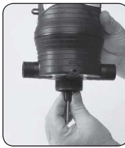
Step 8. Replace #51 SHAFT ASSEMBLY.
