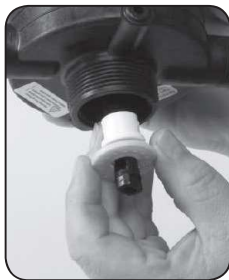
Step 7. Re-install #16 GASKET and #82 SEAL SPACER
