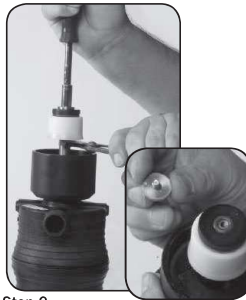
Step 2. Unscrew to unlock and remove #93 CAPSCREW.
