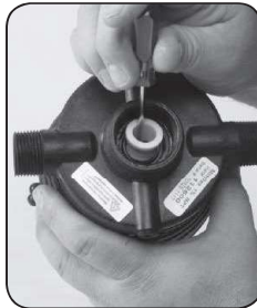
Step 5. Replace #83 SHAFT SEAL SPACER.
