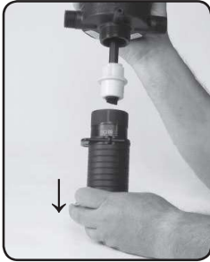
Step 1. Unscrew #7 OUTER CYLINDER from body.
