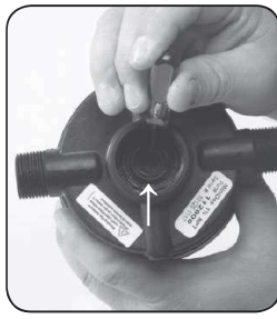
Step 5. Remove #17 O-ring and replace.
