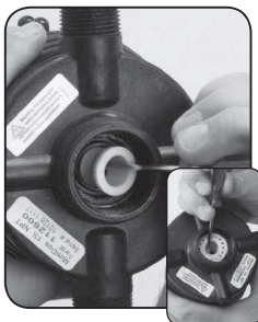
Step 7. Replace #82 SHAFT SEAL SPACER and #16 Gasket.
